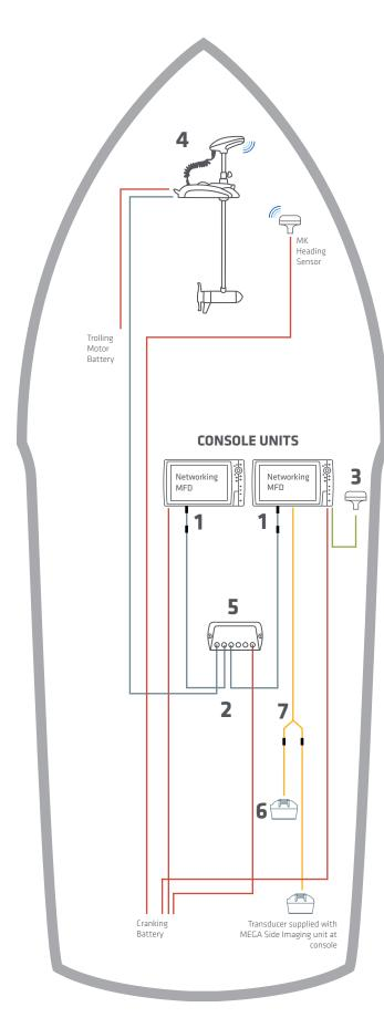
Saltwater - Minn Kota Riptide Trolling Motor with i-Pilot Link and (2) console-mounted Humminbird Units
