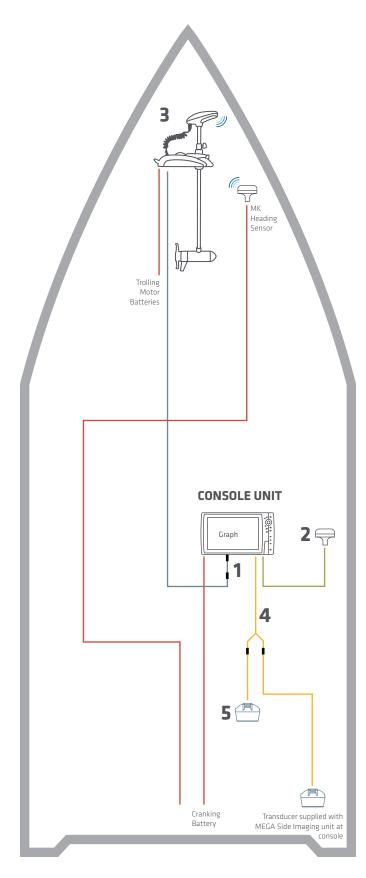
Minn Kota Trolling Motor with i-Pilot Link and (1) console-mounted Humminbird unit
