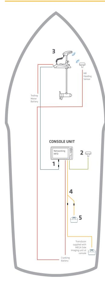
Saltwater - Minn Kota Riptide Trolling Motor with i-Pilot Link and (1) Console Mount Humminbird Unit
