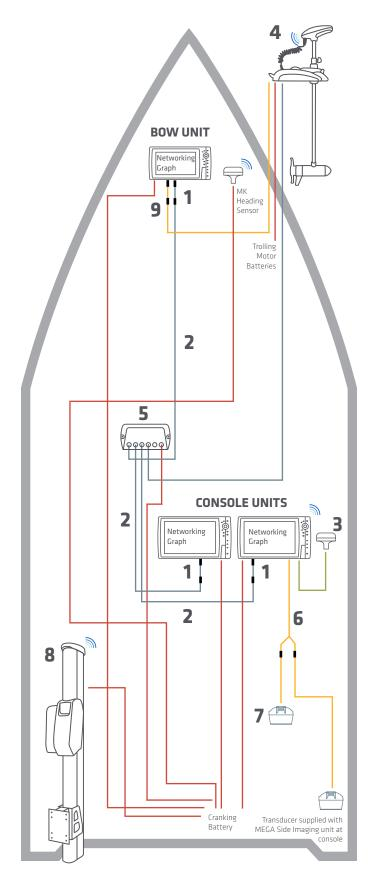
Minn Kota Trolling Motor with i-Pilot Link and Built-In MEGA Down Imaging, (1) bow-mounted Humminbird unit, (2) console-mounted Humminbird units and Talon Shallow Water Anchor
