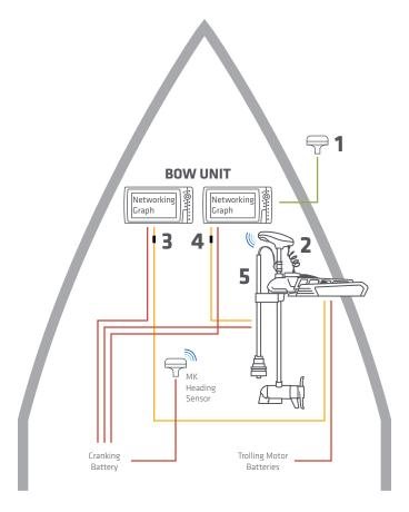
Adding a MEGA 360 Imaging - Ultrex model to a boat with (2) Bow-Mounted Humminbird units and Minn Kota motor with Built-In MEGA Imaging
