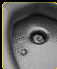
Floor inflation valve with anti-return
